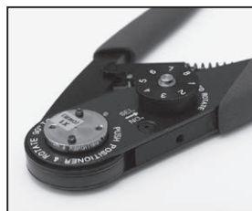
② Tighten with a crimping tool. Dial and adjust depending on the thickness of the wire (1-8).
