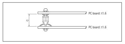
• The dimension C is the distance between the PC boards of 1.6mm that are fit in the both sides of this product.
