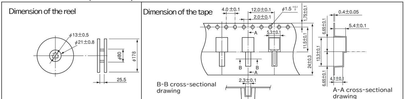
※ The dimension of the reel for HH-51-T is the same as that for HH-5.
