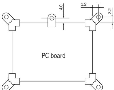
•Please insert EP series underneath to raise 1.5 mm or over from the chassis (base).
