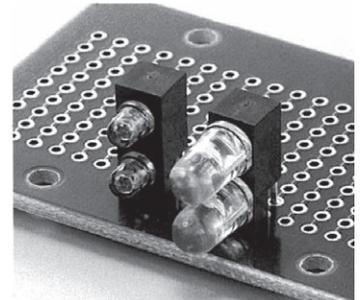
**LED spacer (two-tiered installation type) (three-legged type)**
