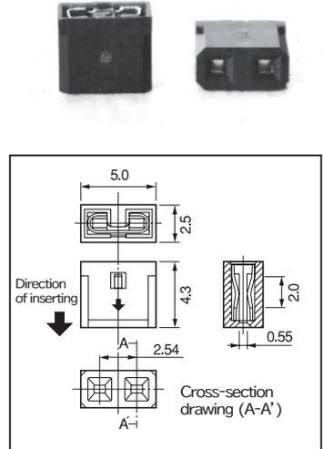
**Jumper socket for wrapping (for the pitch 5.08 mm)**
