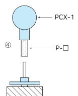
Place it on a flat metal block and press-fit the ring from above by using a tool.
