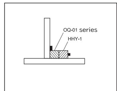
By using OQ-01 series, the SMT boards can be mounted at right angle.
